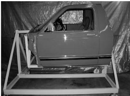
However, we have shown that when a 240 lb. surrogate male is placed in the test fixture and inverted, he is unable to produce adequate force on the press button to release himself from the restraint system. This phenomenon has been reliably reproduced using the test fixture shown here. Additionally, the test buckles used in these tests came from documented production vehicles and had not been modified.
