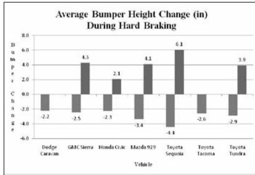
Figure 2: Change in Bumper Height During Hard Braking
