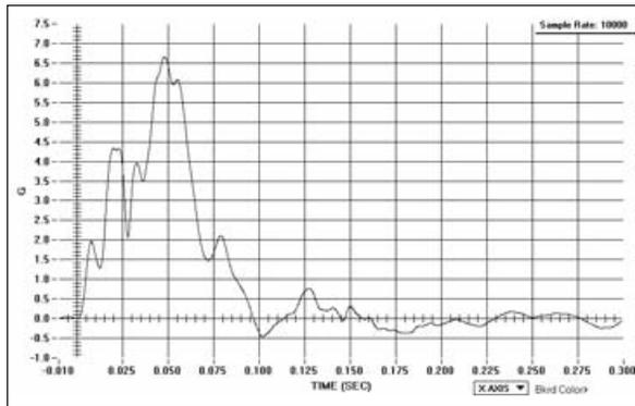
Figure 3: Dodge 5 mph rear bumper to barrier
