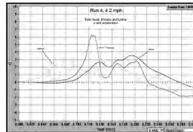
Figure 4: Rider accelerations in Run 4 (4.2 mph)
