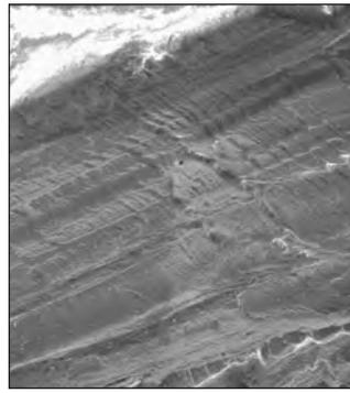
Figure 2: Wallner lines on fracture surface
