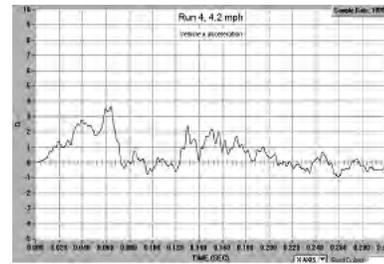
Figure 3: Motorcycle accelerations in Run 4 (4.2 mph)
