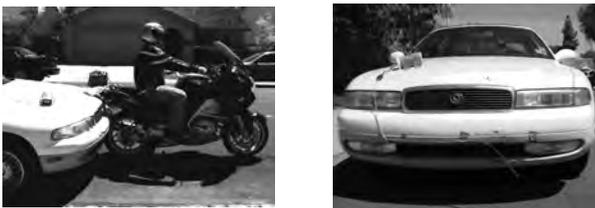
Figure 2: Wheel penetration into bumper and hood to frame contact
