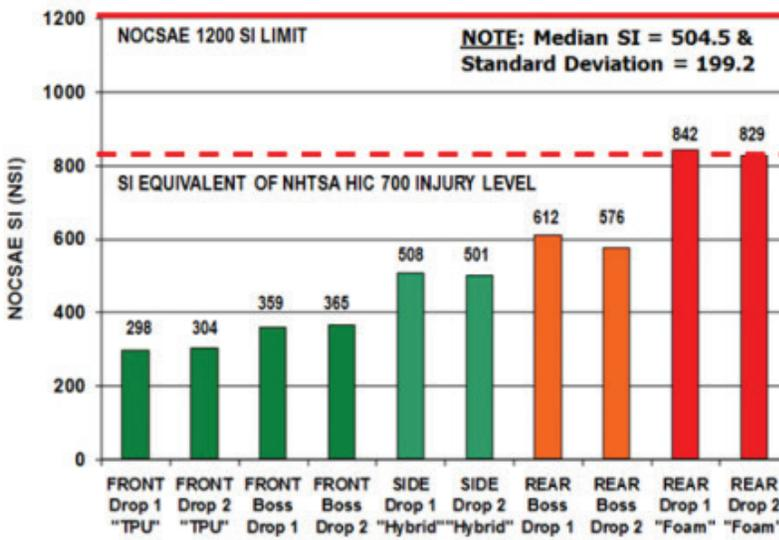
Fig-2. NOCSAE Severity Index Data from 2014 Peewee Youth Helmet Design Approved for Peewee Play
