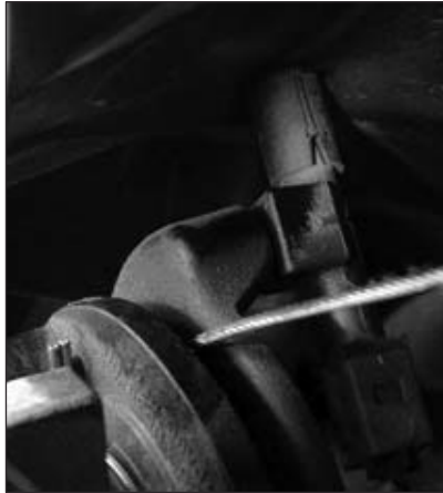
Figure 2: Throttle position sensor entrapment at plastic engine cover.
