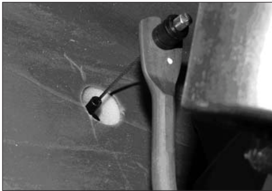
Figure 1: Accelerator cable at firewall and accelerator pedal installation point.
