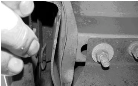
Figure 1: bracket damage in 5 mph rear bumper to barrier
