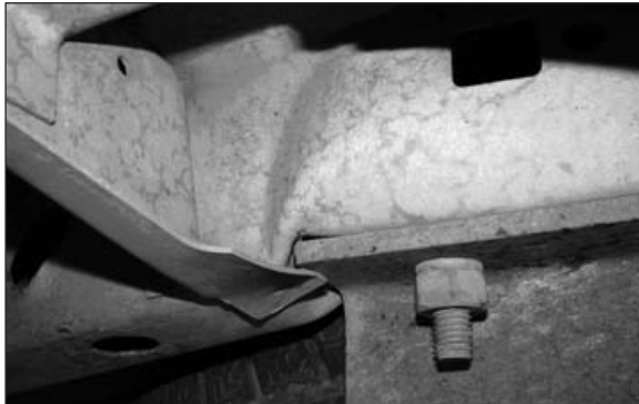
Figure 2: frame damage in 4.7 mph rear hitch to barrier
