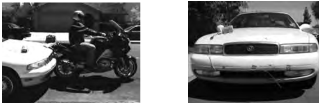
Figure 2: Wheel penetration into bumper and hood to frame contact
