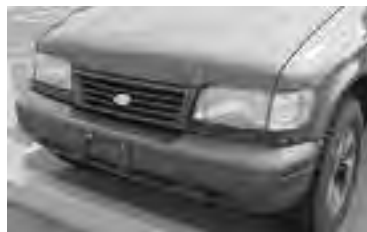
Figure 2, Post Collision Photograph of the SUV. However, inspection of the SUV revealed that there was damage above the front bumper to the left head light and grille areas. In addition, a horizontal rectangular imprint was found on the central front bumper. Thus, the SUV's damage was consistent with a direct contact between its central front bumper and the pickup's rear bumper step. As the
