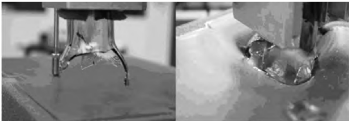
Figure 1: Complex fracture geometry of a broken glass bottle showing the bottle just out of contact and just in contact with silicone rubber/foam skin simulant. The large elastic deflection of the skin simulant is readily apparent.
