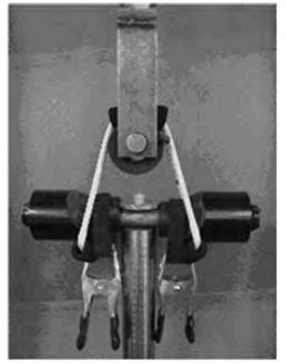
Without any tubing surface artifact, the figure-eight would be expected to eventually break after sufficient repetitive cycles of use, because each cycle will naturally cause a minute amount of degradation of tubing material.
