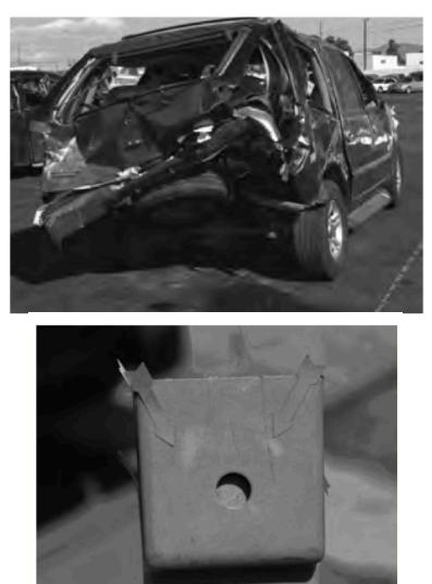
Third Row Outboard Seat Belt Detachable Anchor Compression Testing: Compression tests were conducted on the boot- encased detachable anchor assemblies sectioned from two exemplar seat belt assemblies salvaged from 1999 and 2000 model year Expeditions. The 2000 specimen exhibited more oxidation to the metal plating of the detachable anchor, likely a result of exposure to the elements during storage.
