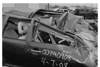
All of the vehicle's windows were fractured during the rollover. Careful examination of the right front seat belt showed approximately 15in of webbing with cut fibers consistent with interaction with fractured glass fragments. However, these fiber disturbances were found on an area of the webbing that would not be exposed to the vehicle's interior if the seat belt was stowed.
