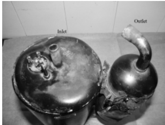
Figure 1: AC compressor showing inlet and outlet.
