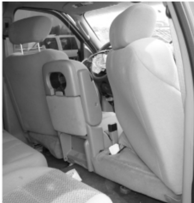
Figure 3. Seat back deformation in pickup.
