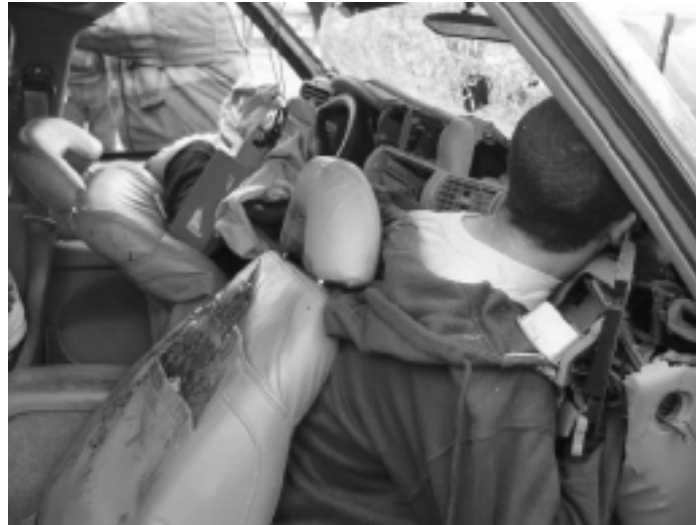
Figure 2. Occupant compartment intrusion in SUV.
