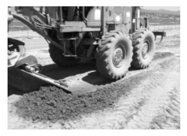
A time-position analysis of the grader at 17mph showed it was approximately 14sec from impact when the tractor was reasonably expected to be in view. Assuming a 2sec perception/reaction time, and allowing 2sec for the grading blade to make soil contact, the grader operator could have stopped in about 125ft. Therefore, it was argued that the grader operator had failed to use precious time available to avoid the collision.
