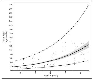
The above graph demonstrates the curvilinear relationship between vehicle delta V and peak head acceleration in 93 human volunteer crash tests. The shaded section is the 95% confidence interval, and the dotted line is the predictive interval depicting the likely range of accelerations in the general population.
