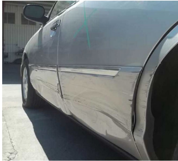
Figure 6: Example of closing of body panel gaps.
