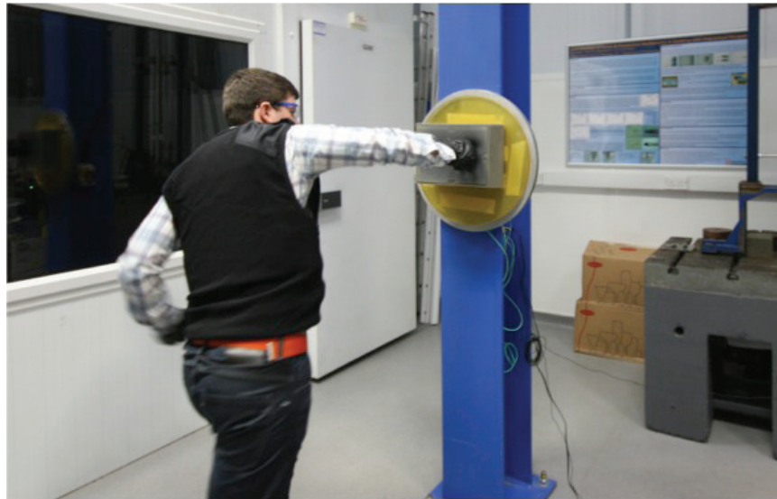
Figure 1: A volunteer performing a stab into the dynamometer. Force data is taken from three load cells and the system was calibrated with known applied forces to ensure the peak forces that were recorded were accurate.
